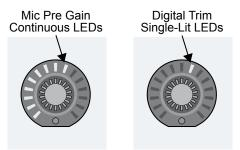
The gain for the selected channel can also be adjusted from the Overview touch screen. The Digital Trim control that is normally displayed is now replaced with a Gain knob showing a readout of the amount of gain being applied by the mic preamp. Note that the displayed value takes into account whether or not the 23 dB PAD is engaged. So what you see is what you get; no subtraction required (see, we're always striving to make your life easier!). The gain range is summarized below:
